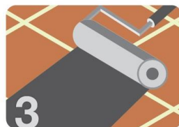
3 Apply Crocodile Flex Shield on the original tiles before retiling
