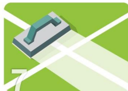
7 Leave for 24 - 48 hours before using the correct Jorakay grouting. Use the trowel to fill the grouting groove (swipe diagonally). Leave for 72 hours before opening the area for use.
