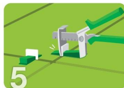
5 Level the tiles with Crocodile Tile Leveling System
