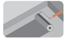
4.After the first layer is dry (after 4 hours) paint the second layer of sealant. Paint 10 cm up the wall from the base.
