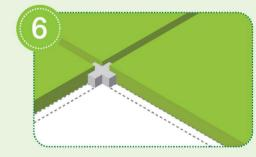
Use a spacer and allow at least 2 mm for grouting.
