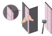
**Application** Put the tile attach to the trim, press it or tap with rubber hammer along the trim. Then, start the second roll until the space is filled. Then, follow the grout process.
